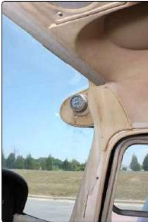
**Figure 10-67.** A bimetallie outside air temperature gauge and its installation on a light aircraft.
