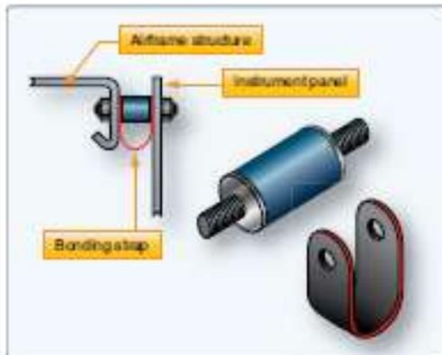
Figure 10-133. Instrument panel shock mounts.
