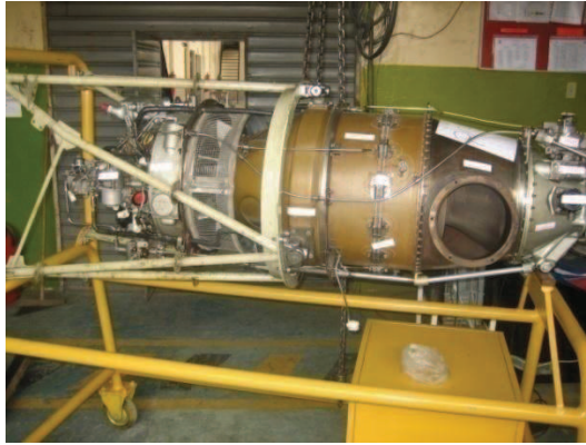
Figura 7. Motor PT6-34 (inoperable)
