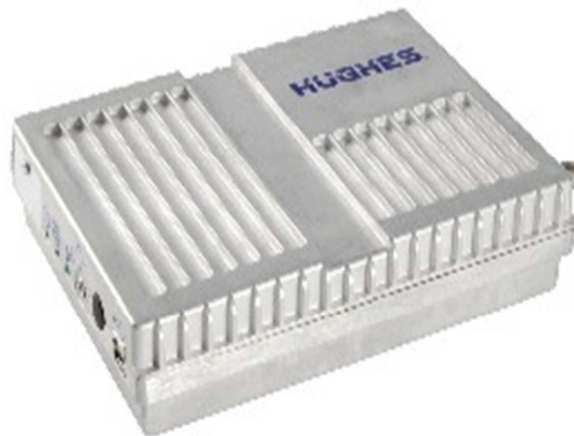
Figura 2.19 Antena BGAN Hughes 9502
