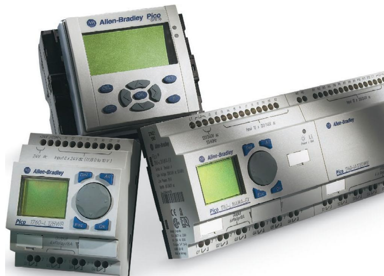
FIG. 1.3: Nano PLC, Allen Bradley 3
