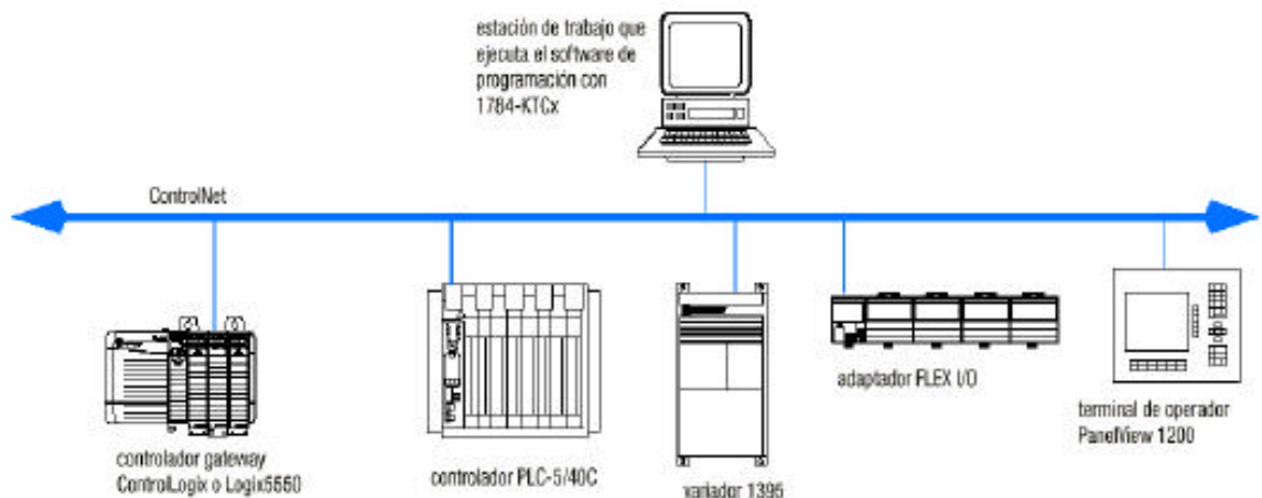
FIG. 1.49: Red ControlNet, Allen Bradley
