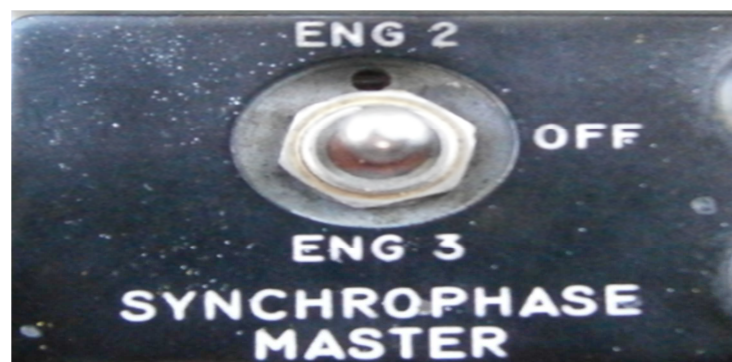
Figura 2.25: Interruptor maestro C-130H.
