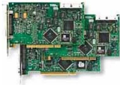
**FIGURA II.81** Tarjeta NI PCI-6024E
