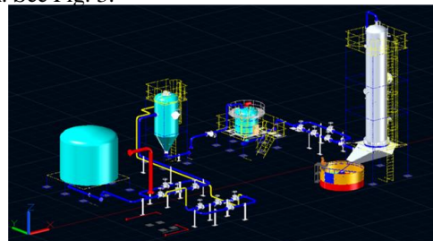
Figure 3. Ammonium nitrate granulation plant design.
