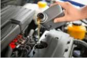
A close-up photograph showing a person's hand pouring dark oil from a grey plastic can into the oil filler neck of an engine. The engine components, including the oil cap and various hoses, are visible in the background. |
