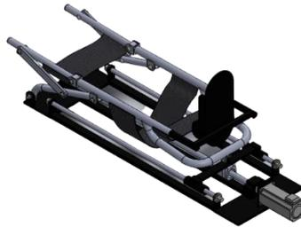
**Fig 6.** Mechanical prototype for knee rehabilitation.
