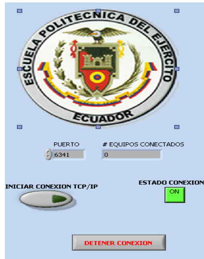
Figura 2.9.2. Panel Frontal servidor TCP/IP.
