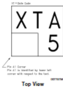
LM358TP micro SMD Marking Orientation
