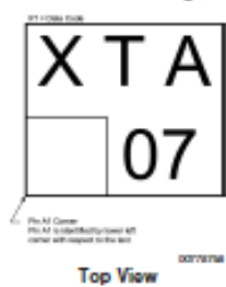
LM358TP micro SMD Marking Orientation
