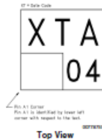
LM2904TP micro SMD Marking Orientation
