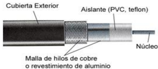
Figura 1.16: Cable coaxial
