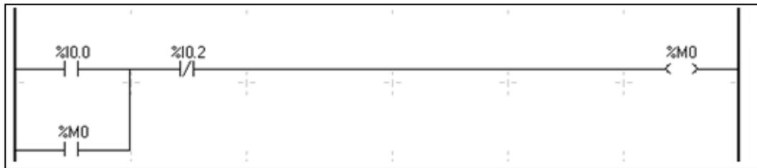
**Figura 2.16 Ladder Logic del PLC Twido**
