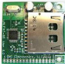
μALFAT-SD is an OEM board of μALFAT™ chip. The low cost and the ease of use, makes μALFAT-SD the ultimate solution for OEMs and hobbyists.
