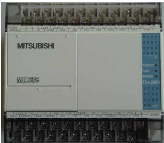
Fig. 4.104 PLC MITSUBISHI FX1S-30MR 29
