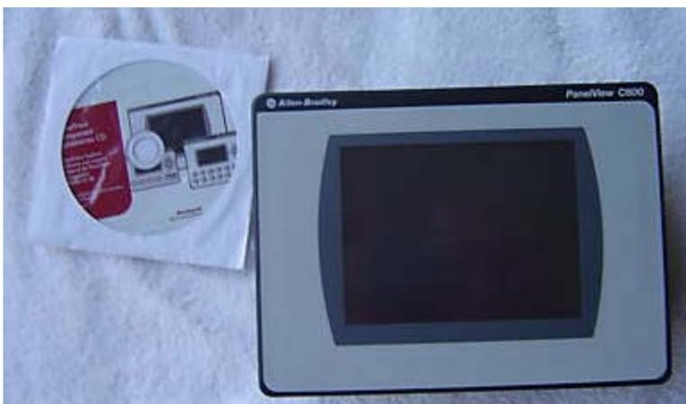
**Figura3. 14** Panel View Component C600
