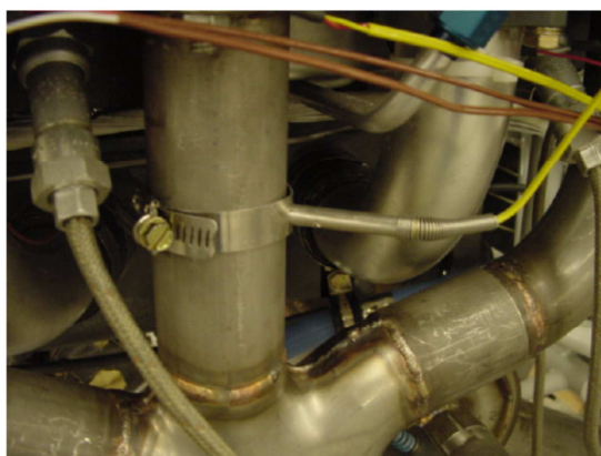
EGT Probe Location
