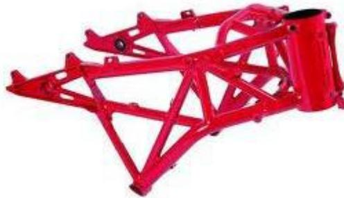
Figura 2.8 Chasis multitubular triangulado
