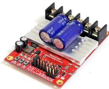
Figura 2.76: Tarjeta de control Roboclaw 2x15A 134 .
