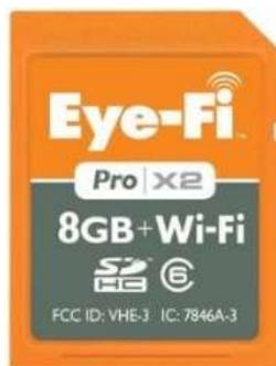
**Figura 2.49. Tarjeta Wi-Fi Eye-Fi Pro X2.<sup>38</sup>**
