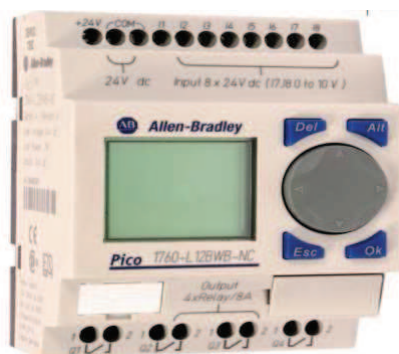
Figura 115. PLC Allen Bradley pico 1760
