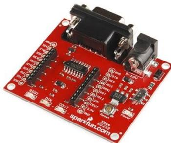
Figura 2. 10 Xbee Explorer RS
