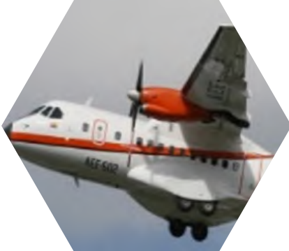
Type: CASA CN235-300 Max Speed: 450 km/h Weight (kg): 15,500 Year: 1988 Capacity: 48 pax
