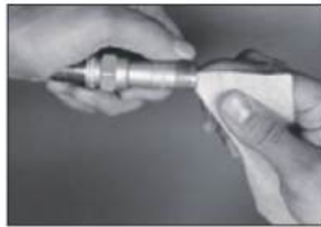
Connector seats may be cleaned with fine-grained garnet or sand paper.
