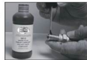
Applying anti-seize compound.
