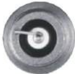
Spark Plug Fired Positive Adverse Ground-Electrode Wear
