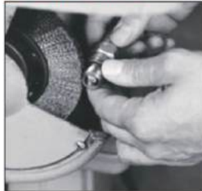
Cleaning threads with a rotary brush.
